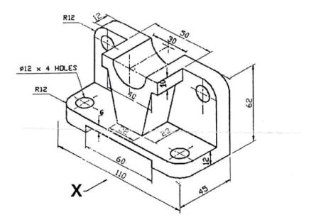
9. The figure shows the side view and front view of a machine Block. Draw the isometric view of the block.
